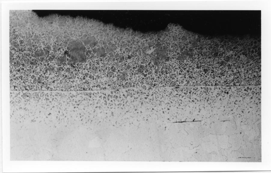
Plate 1. Tapered bar SF1590. Specimen from wide end showing ferrite grains (pale, lower) and pearlite (dark) at the metal surface (black, upper). Across the centre (left to right) is a light-etching weld line. Nital etch.
