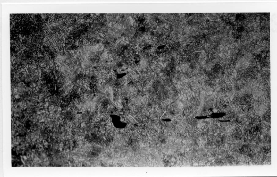
Plate 4. Bar SF1594, showing high-carbon steel of eutectoid composition at the bar end. Pearlite (dark), glassy inclusions (black). Nital etch.
